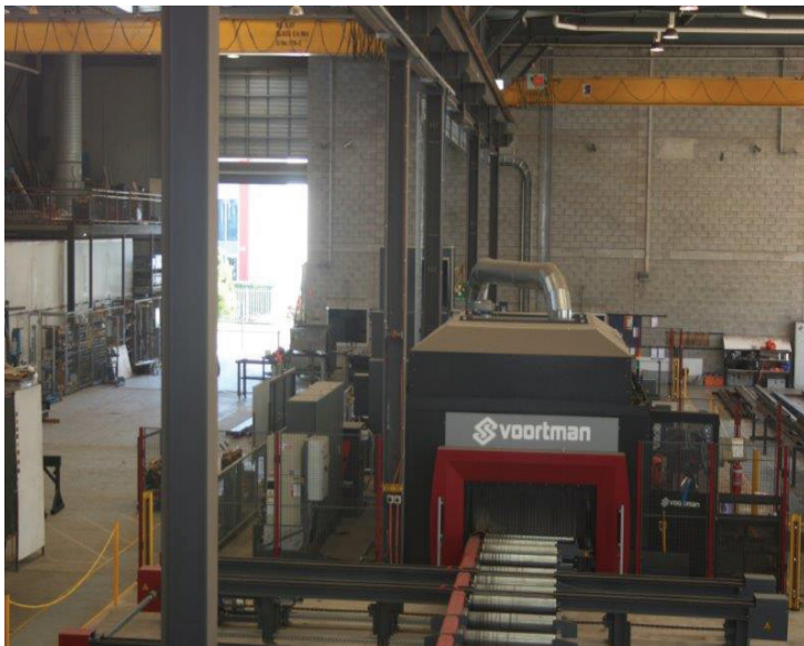
Voortman V808 Coping Machine to fabricate, cut and mark the steel
